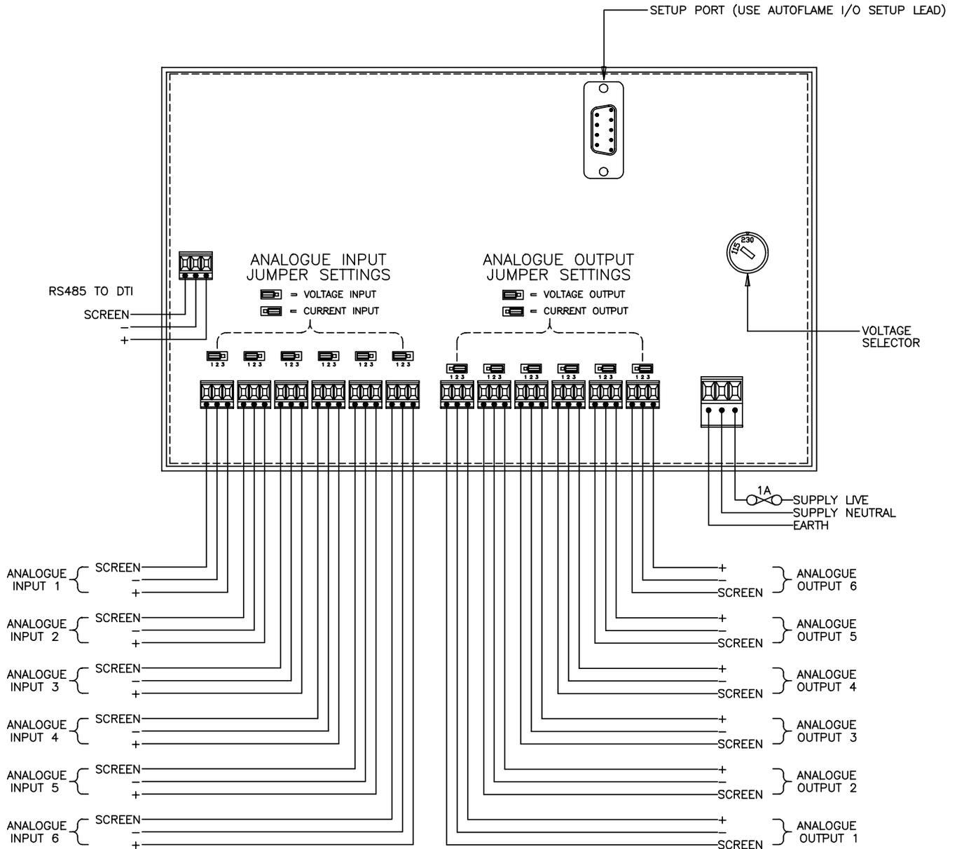
**6.14.7 M.M. to Analogue Input/Output Unit Connection Diagram**
