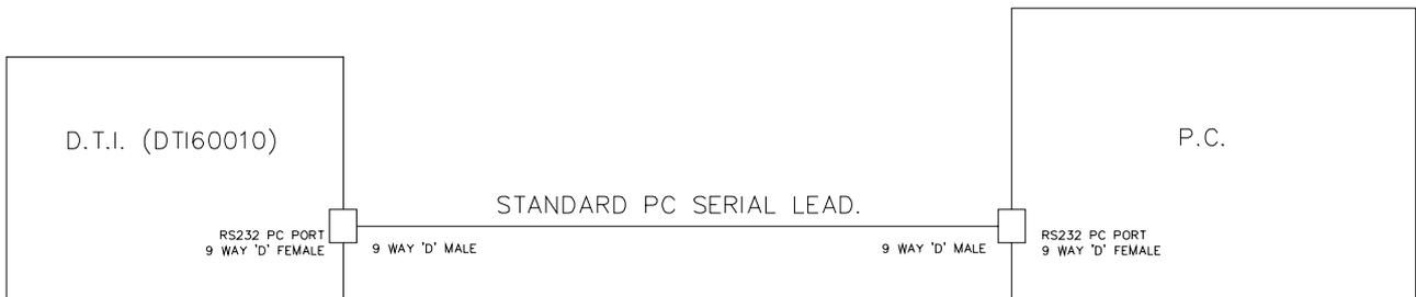
**PC-DTI Cable (for older DTI units that do not use a standard PC serial lead)**
