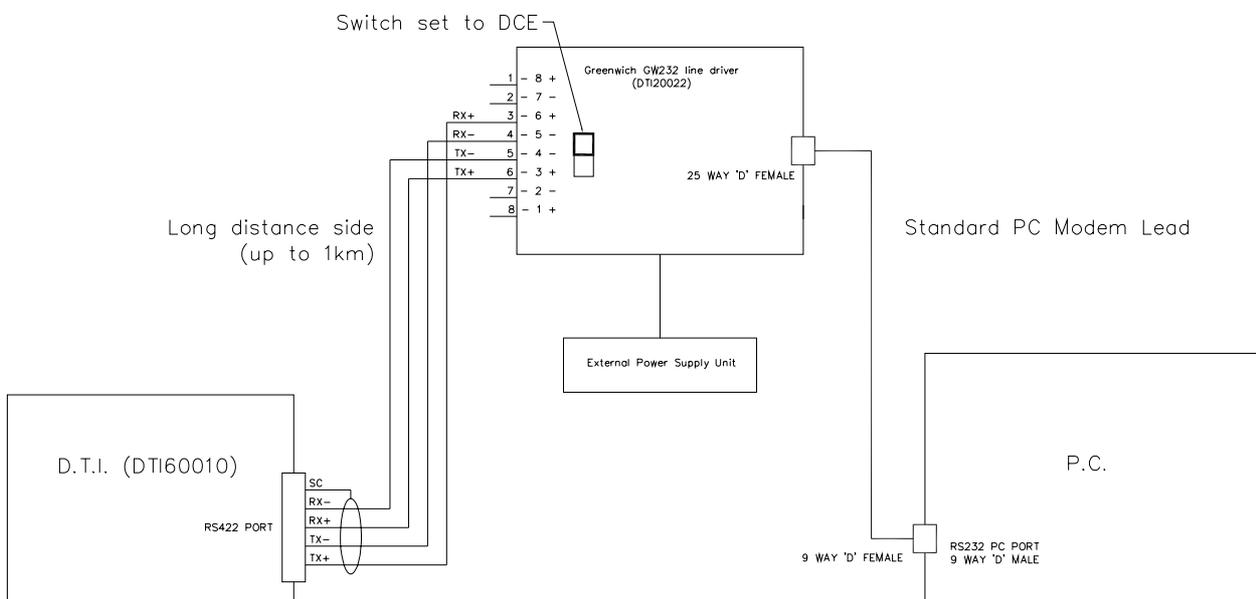
Example shown using line drive type GW232F made by Greenwich Instruments Limited.
